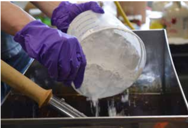
Store and handle diatomaceous earth (DE) carefully. If this filter aid gets damp or musty, it can impart a musty flavor to your syrup. The safe handling of DE includes taking precautions to avoid inhaling the DE particles.
