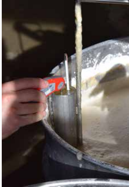
Syrup cools rapidly in a hydrometer cup. Take the density measurement immediately after reading the syrup's temperature and then apply the proper correction depending on the value.
