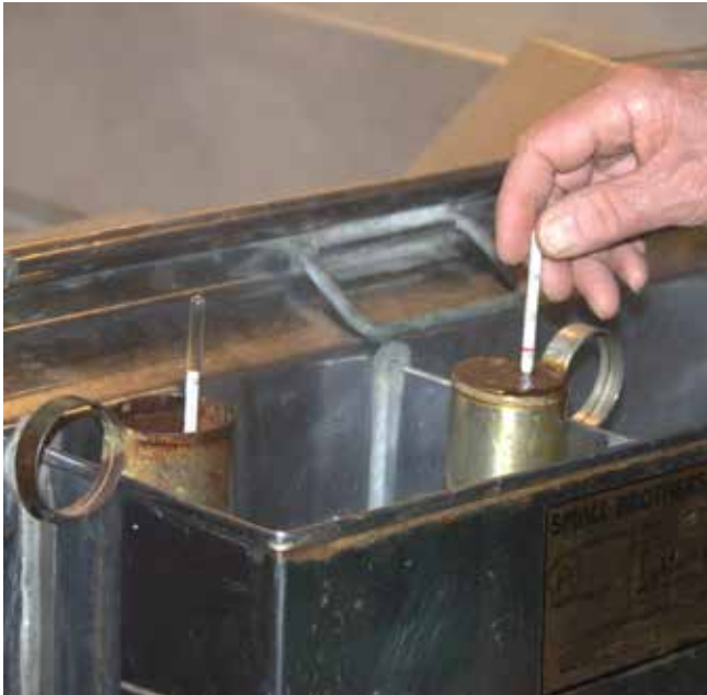
Lower the hydrometer into the cup gently, so it doesn't break. Have at least one spare, in case it does.
