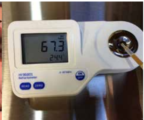
Optical and digital refractometers are excellent tools for testing the density of syrup.
