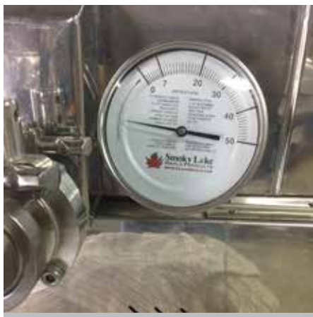
A thermometer that goes into a fitting in the evaporator pan can be quite handy. One that can be adjusted to accommodate changing boiling temperatures even more so.
